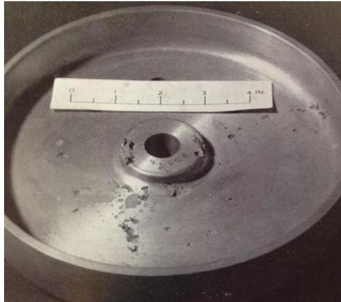
This type of blow hole is unique in appearance as it consists of small holes with rounded or irregular shapes which may at times contain shot/grit at or just below the casting surface. These blowholes mainly occur particularly on top surfaces and below cores. They may be revealed on cleaning or after machining. These holes have discoloured surfaces which are often associated with slag inclusions and sand grains.
