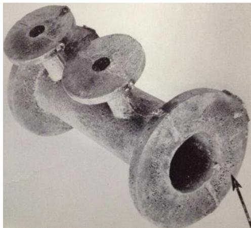
Localized areas of small cavities/pits on the surface of the casting. The picture on the left shows defects on the flange of a 4'' bore branch pipe in Ni-Cr Iron alloy cast in dry sand. This defect usually occurs on heavier sections of castings which solidify at a slower rate than the thinner sections. Rule of thumb suggests that it is most commonly experience on castings ½'' and over. Stainless and other high alloyed steels are susceptible to this defect.
