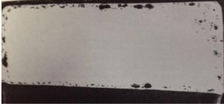
Small cavities adjacent to the surface of the casting (and usually on all surfaces of the casting). In many cases the surface of the casting appears to be normal (which makes this a difficult defect to identify in the as cast condition). In some cases however, surface pitting may be present as illustrated below:
