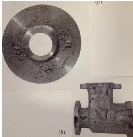
Localised patches of round or irregularly shaped cavities of significant size. The walls of the casting are smooth and often coloured with oxidation tints. The two examples on the left represent:
